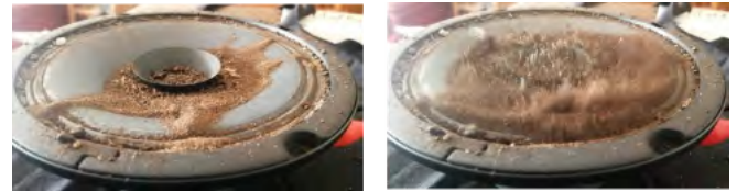
Fig. 4. The soil vibrates above the loudspeaker in Fios de Silere.
