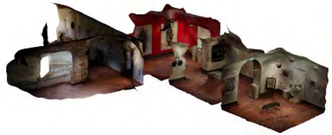
Fig. 2. 3D rendering of the exhibition rooms and adjacent corridor. The scan was taken with cameras equipped with LiDAR sensors and a Polycam app (Source: authors ).
