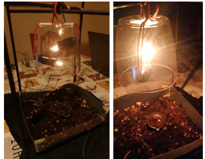
Fig. 2. Prototype a top structure with an inverted plant table and a small speaker.
