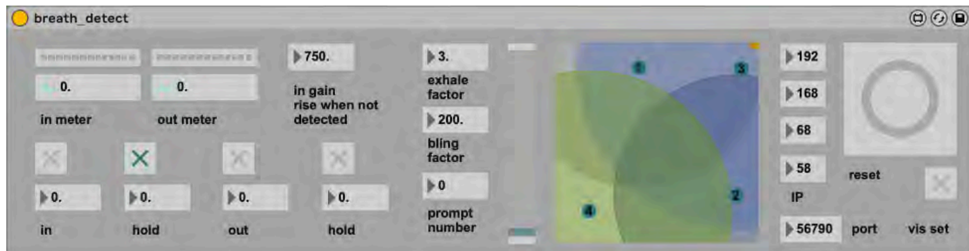
Fig. 4. Interface panel for breath detection. It comprises the illustration of the breathing phase, the relative amount of air in the lungs indicated by the fader.
